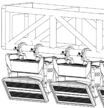
Two quarter-turn brackets are supplied with the fixture if it is to be flown above the ground. Rig the fixture to a support truss or structure using the supplied brackets and suitable clamps.
