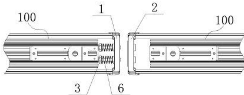
(Insert both Pins to connect the devices)
