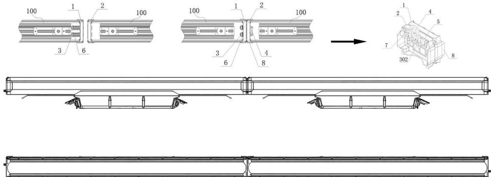
For the first uses this may be a little hard. Move the devices a little until the Bolts can be inserted completely. For vertical installation do not exceed the amount of 4 pieces. (caution, provisional specification) In case of hanging installation, each device needs to be saved individually! Using the quick-release pins for horizontal installation is not recommended. Each device should individually be installed with the given installation options below.
